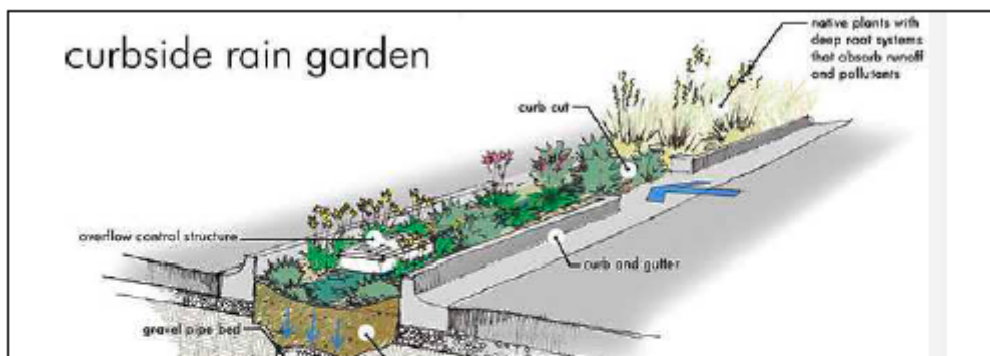
Figura 19 – Schema rain garden
